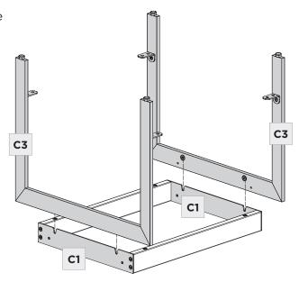
Thread the remaining 4 Screws (H2) into the holes in the **Legs (C3)**.
