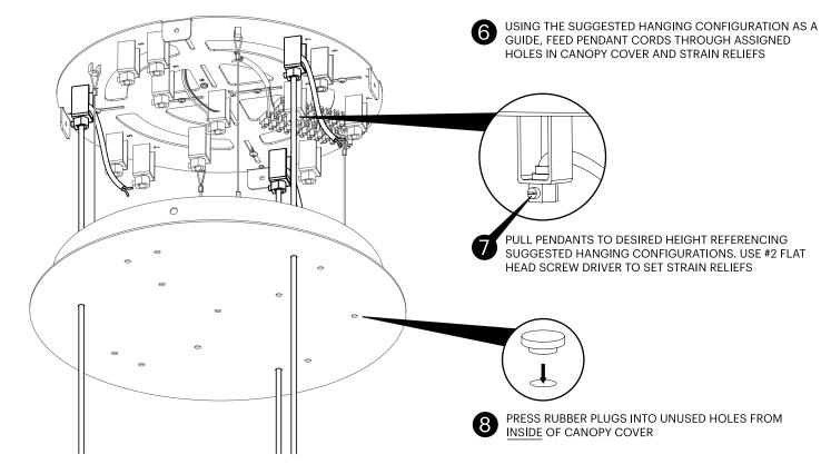
NOTE: INSTALLATION SHOWN IS FOR BOLA SPHERE CHANDELIER 3. FOR BOLA SPHERE CHANDELIER 5 AND 7, FOLLOW THE SAME WIRING PROCESS USING THE HOLE PLACEMENT OUTLINED IN SUGGESTED HANGING CONFIGURATIONS.
