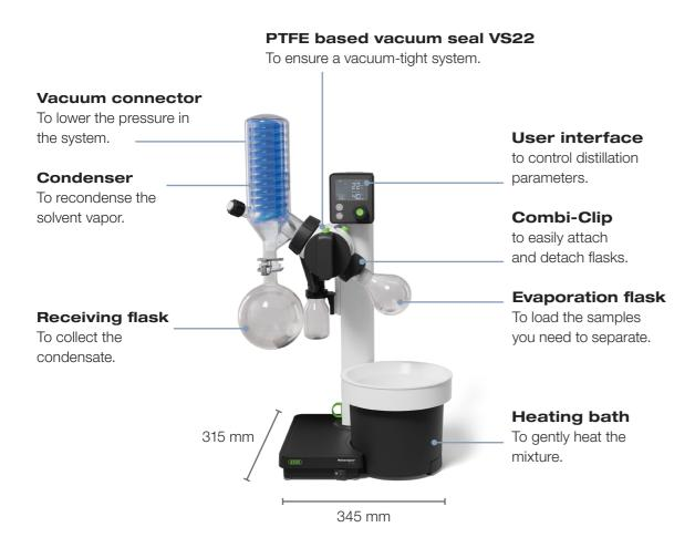
Rotary evaporation is an essential and gentle method for many laboratory applications, such as:
