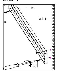
Position bracket to wall at desired location and fix bracket to wall with screws. \*Use screws required depending on wall type.
