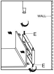
Position shelf metal holes at rear over the bracket holes and screw in 4 screws to top and bottom.
