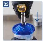
Select the right adapter, align the spray gun with the arrow and push down until firmly in place.
