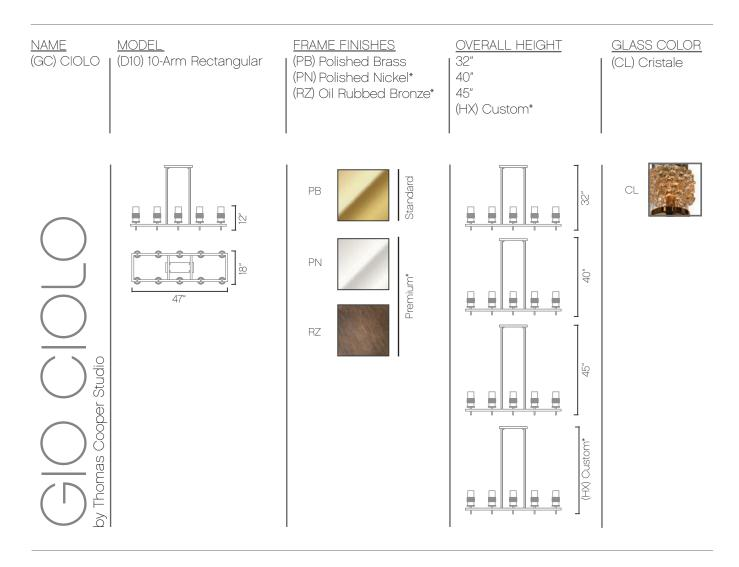
Lamping: D10 (10) 25-60W E12, 120V Dimmable (LED and Antique style Edison bulbs available) UL listed (or equivalent) for dry location
