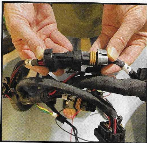
The Holley Terminator X Max will work with the factory wideband oxygen sensors, but the Holley Dominator needs a companion wideband sensor (PN 554-100 NTK). The sensors plug in via this harness.
