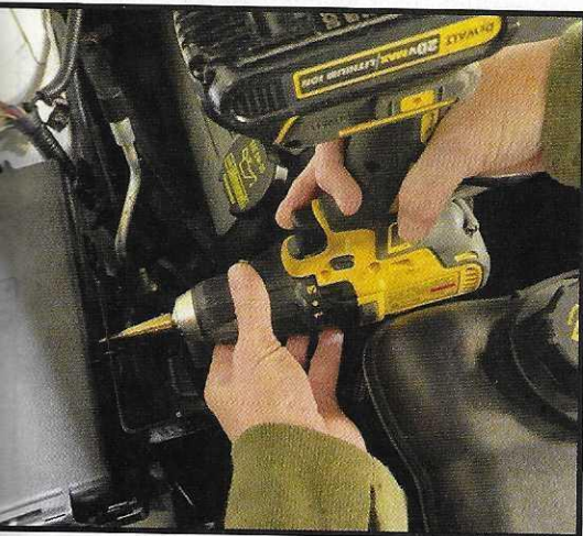
The Holley EFI controller is not a direct replacement for the factory controller, it will fit on the same bracket. All that is necessary is drilling a small hole in the bracket.
