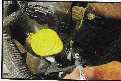
While unplugging the factory wiring connector at the engine control module, he marks the center plug with a permanent marker to ensure that the connectors don't get mixed up when plugging them into the Gate-Way.
