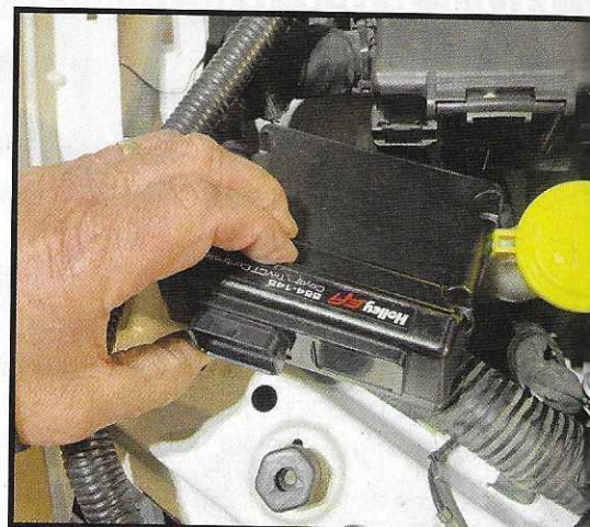
Enabling control of Ford's Twin Independent Variable Cam Timing, Holley offers an add-on TIVCT controller box that plugs into its EFI system. Anderson plugs this unit into the harness and slips it under the fuse box.
