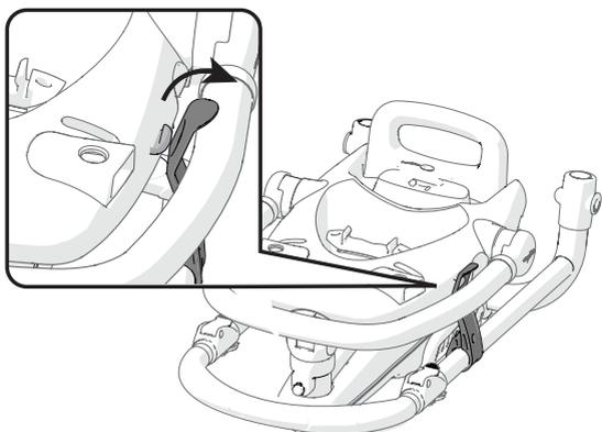
Release the latch on the side of the frame.
