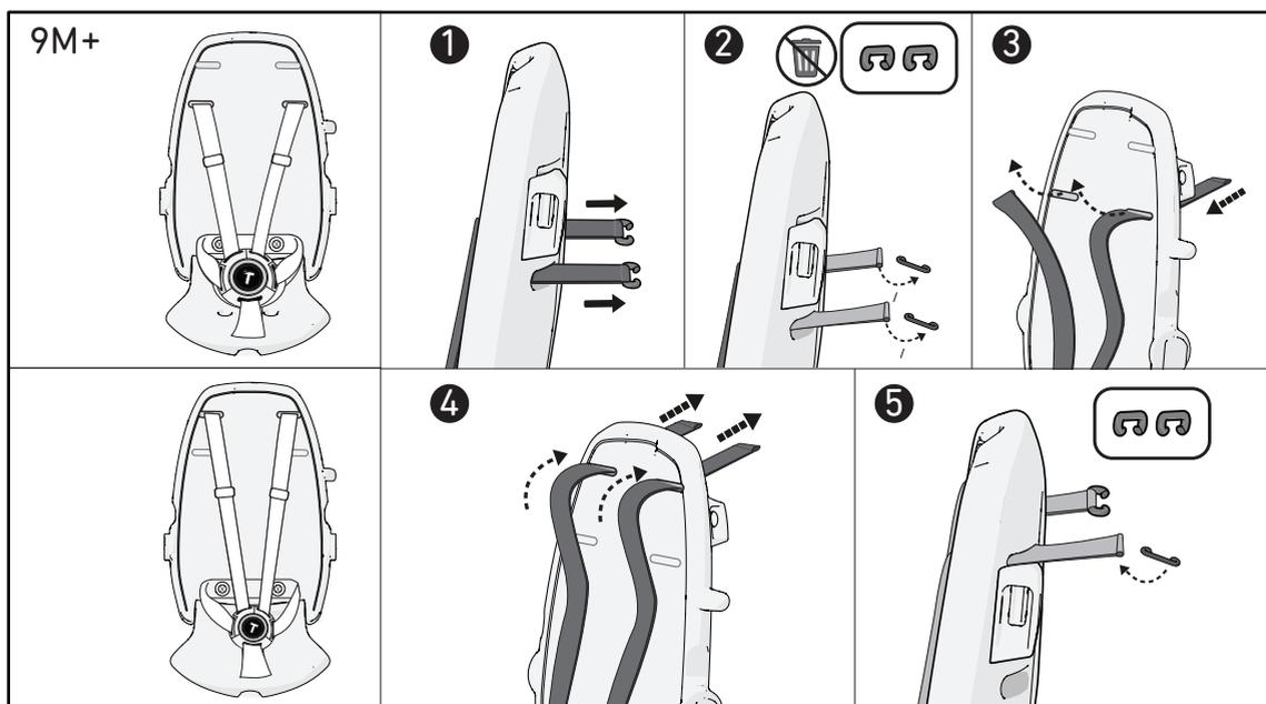
2. Release the plastic parts attached to the straps.
