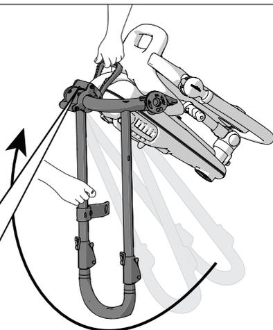
Rotate the parent handle in the direction of the arrow until it clicks into place.
