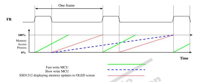
The starting time to write a new image to OLED driver is depended on the MCU writing speed. If MCU can finish writing a frame image within one frame period, it is classified as fast write MCU. For MCU needs longer writing time to complete (more than one frame but within two frames), it is a slow write one.
