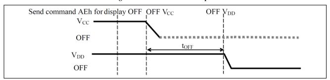
Figure 6-17: The Power OFF Sequence
