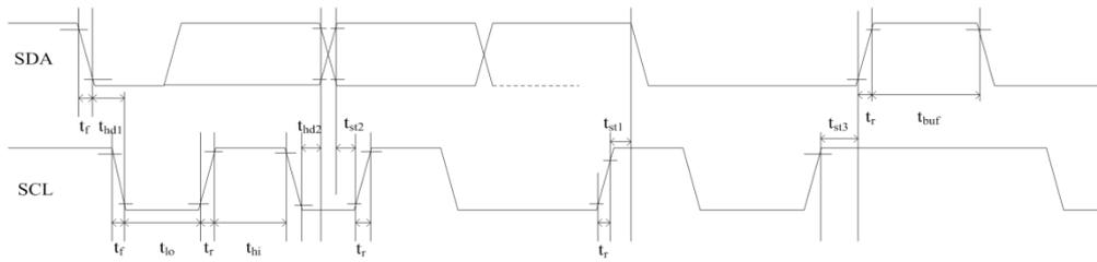
**Test condition 1: 1.8V host interface voltage, 400Kbps transmission rate, 2K pull-up resistor**
