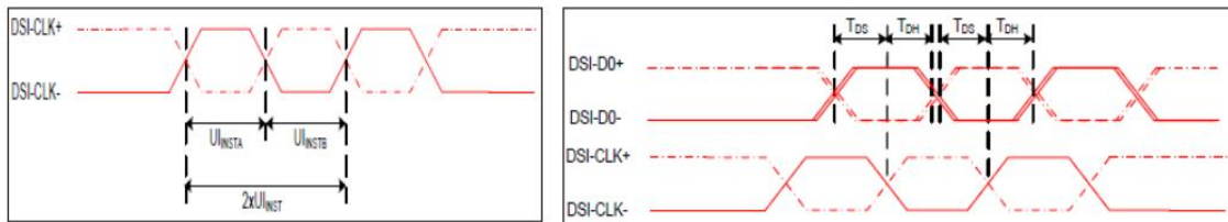
DSI clock channel timing
