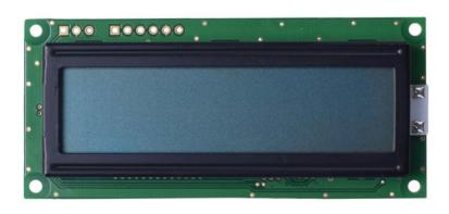
DM-LCD1602-401 1602 SERIAL CHARACTER LCD WITH 12C, SPI OR RS-232(TTL) INTERFACE
