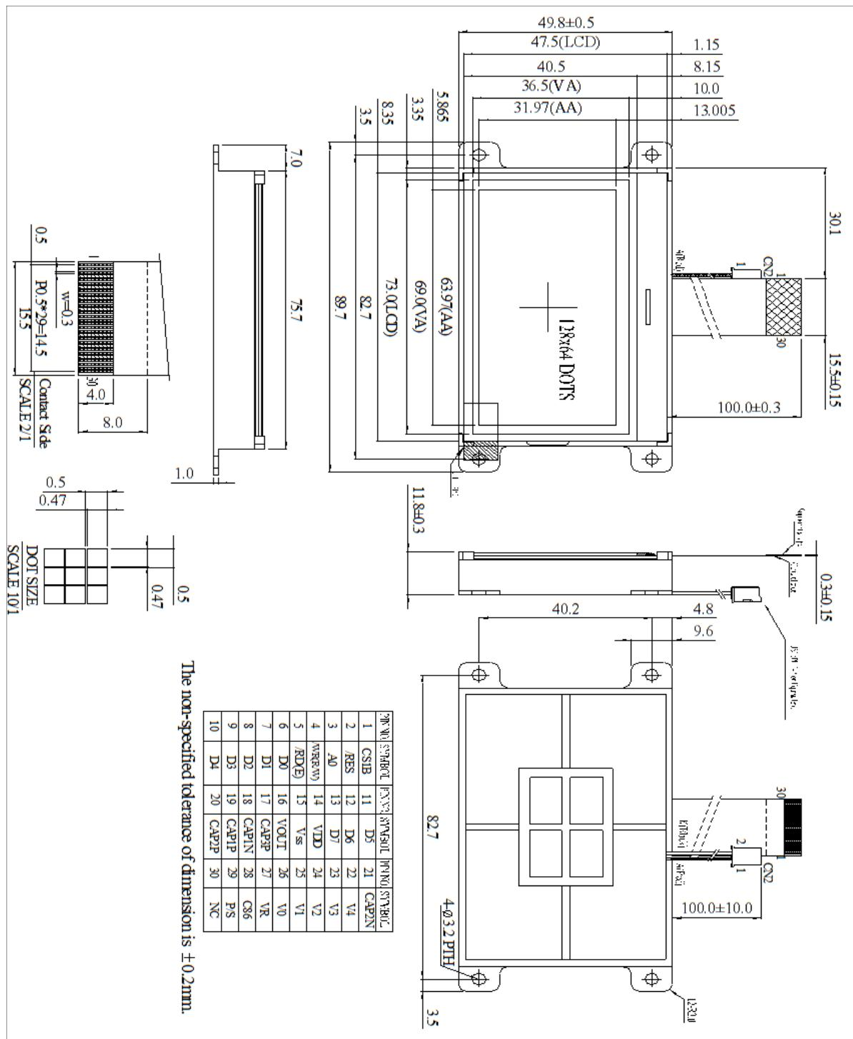
The non-specified tolerance of dimension is  $\pm 0.2\text{mm}$
