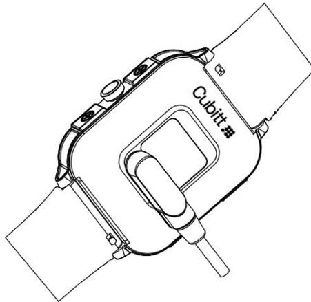
Connect and charge the watch according to the picture. It needs to be charged to activate the watch when it is started for the first time.
