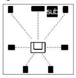
As explained on page two under "Subwoofer positioning" you have various choices. The above illustrations are the optimal placements of both loudspeakers and the Subwoofer.
