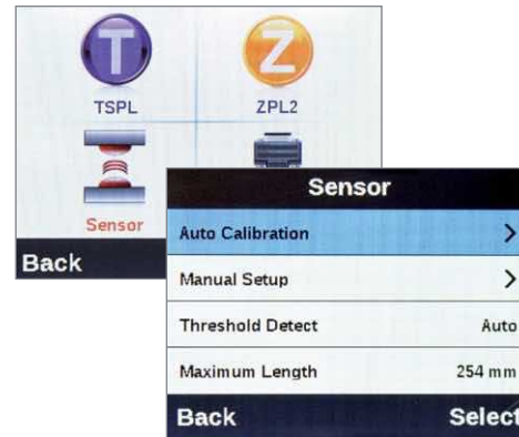
Step 2: Calibrate via Full Colour LCD Display
