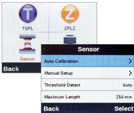
Step 2: Calibrate via Full Colour LCD Display
