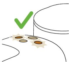
**12 When the flushing cycle has finished, the small drink and large drink buttons flash a few times.**
