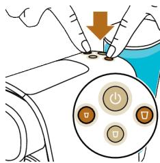
8 The small drink button starts to flash quickly. Press the small drink button to activate the descaling cycle. The system dispenses the entire descaling solution at regular intervals. This takes up to 30 minutes.
