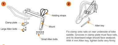
Mounting bottle cages. Tighten bolts firmly.
