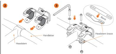
Position clamp on middle of handlebars, facing front, button-side up (rubber shims should be flush with clamp arms and sit flat on handlebars).
