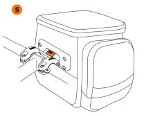
Push bag down, sliding it until it locks into mount. When bag is attached correctly, there should be a distinctive 'click' sound.
