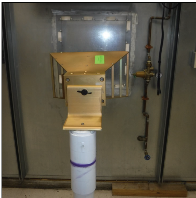
Photograph 17. Shielding Effectiveness, SmallHorn, Vertical, Isolation
