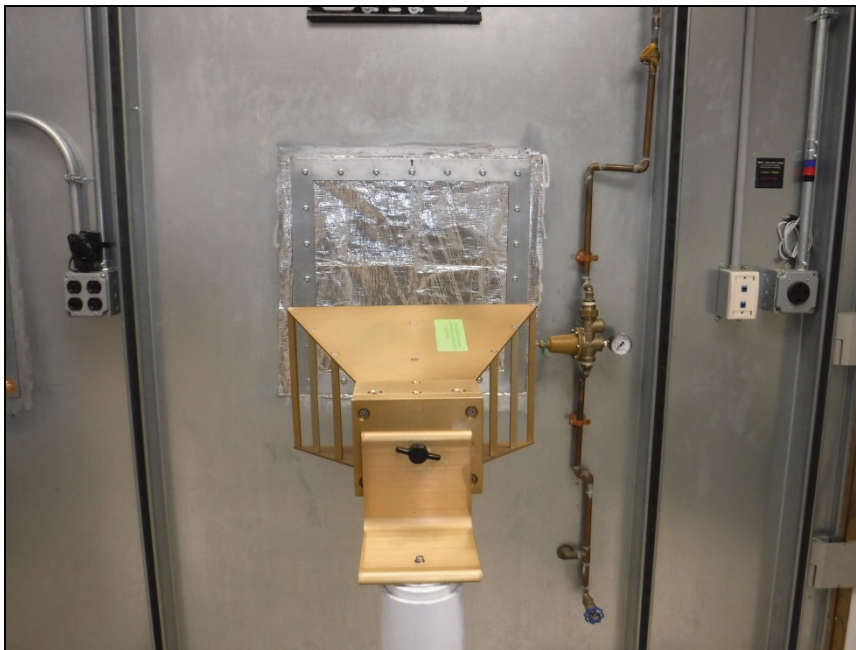
Photograph 15. Shielding Effectiveness, SmallHorn, Test
