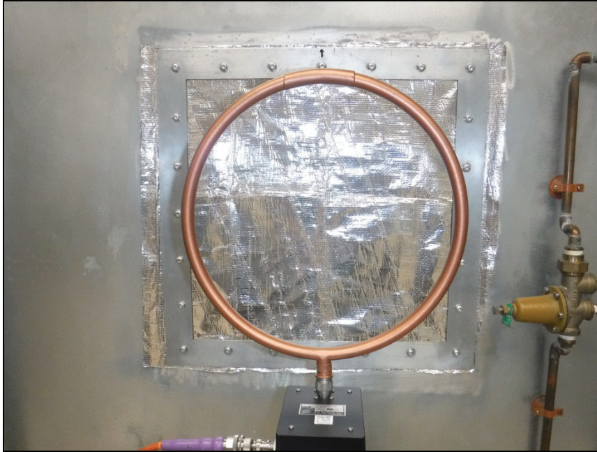
Photograph 12. Shielding Effectiveness, Loop Test
