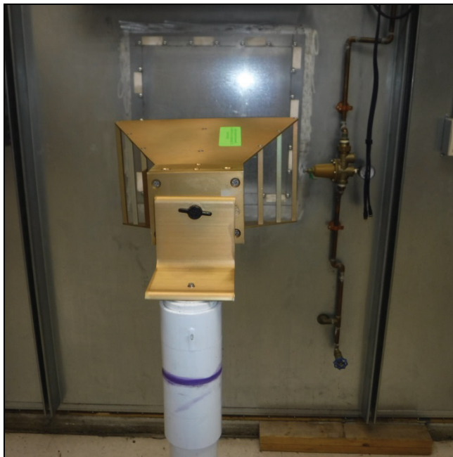
Photograph 17. Shielding Effectiveness, SmallHorn, Vertical, Isolation
