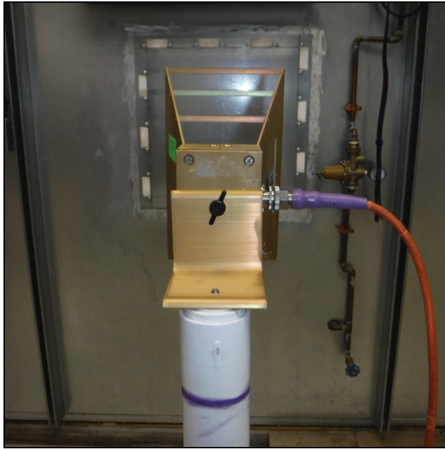
Photograph 14. Shielding Effectiveness, SmallHorn, Horizontal, Isolation
