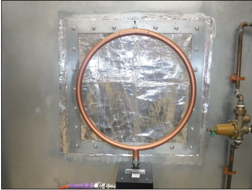
Photograph 12. Shielding Effectiveness, Loop Test
