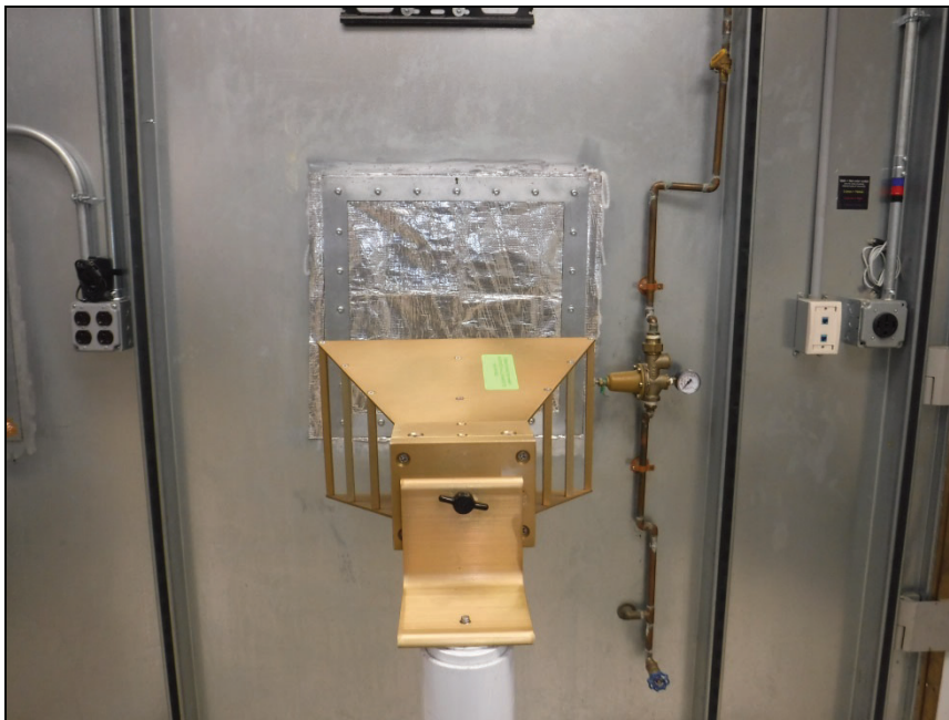
Photograph 15. Shielding Effectiveness, SmallHorn, Test
