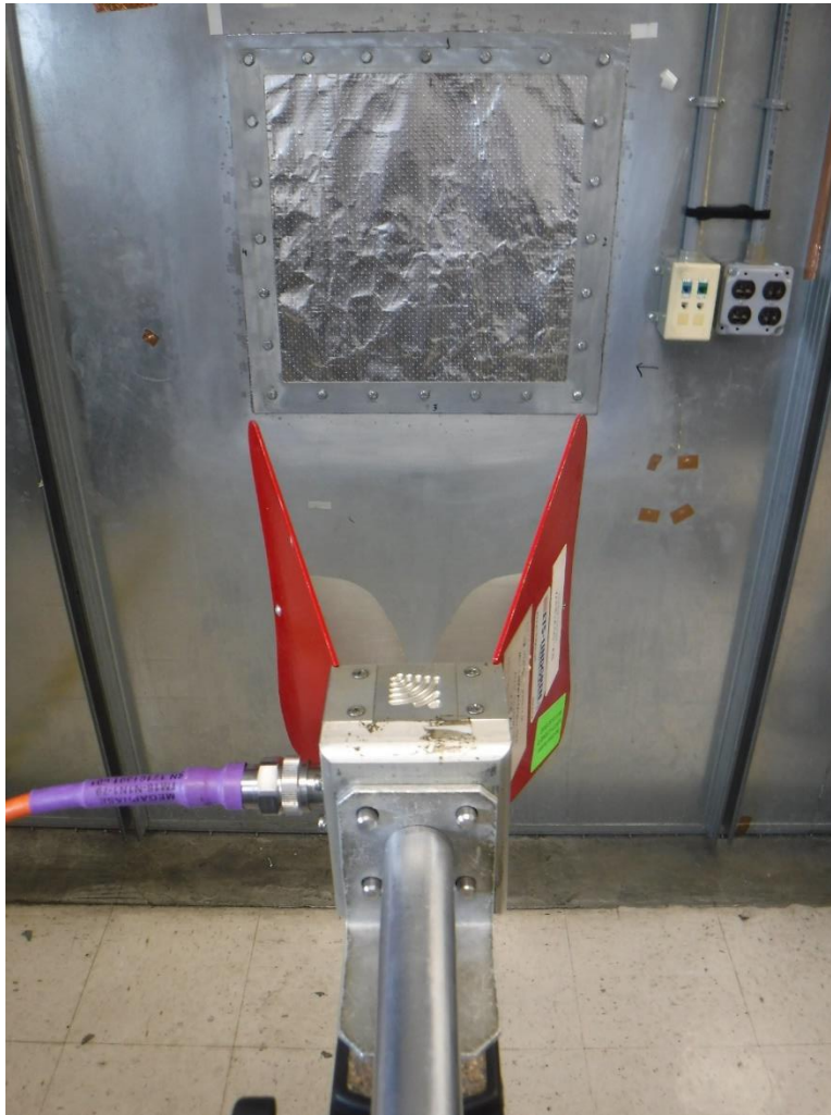
Figure 18: Test Sample (Horn Antenna Horizontal Tx)
