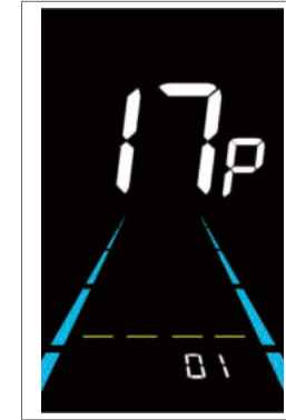
Controller cruise control setting interface
