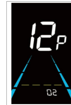
Pedal assist Start-up intensity setting interface
