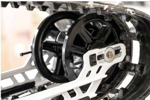
5. Install Tough Wheels onto rear skid in stock location. Use new  $\frac{3}{8}$ " bolt, nut and washers to bolt onto skid. Align track adjustment collars and bolts. Tighten but do not torque until track is readjusted and aligned. Use the following guide to properly adjust track.
