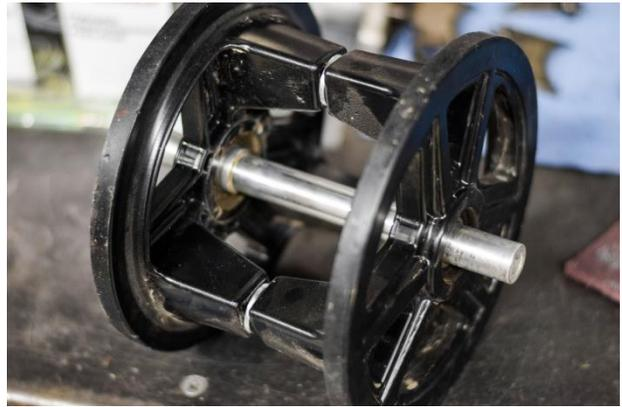
4. Bolt second Tough Wheel onto stock axle as shown. Tighten connector bolts
