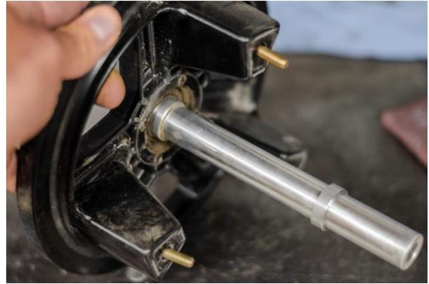
2. Install the stock axle onto the new Tough Wheel. Install the three wheel connector bolts as shown.
