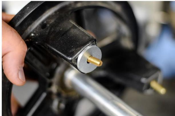
3. Install spacer onto connector bolt as shown.
