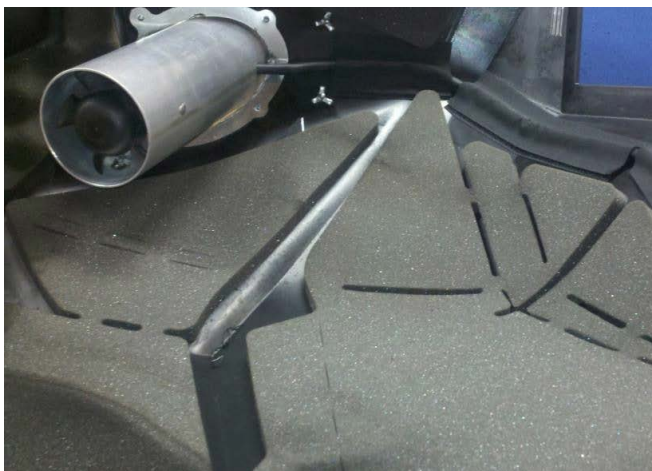
15. Clean the area where the tape is about to be affixed thoroughly with isopropyl alcohol. Clean it 2 or more times to ensure that the surface is clean. Let it dry completely, and then apply the tape. Make sure that the tape is close to the foam near the top edge to allow clearance for the wire when the panel is reinstalled. Route the wire inside the hook and loop as shown.
