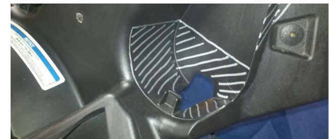
16. Remove spare belt from clutch cover and mark as shown. Take care to reference from the picture to ensure you know what to cut. Lined area is to be removed. Pictures continued on next tile..
