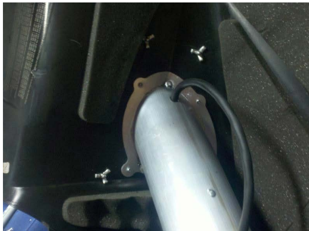
13. Placing the fan motor assembly on the inside rivet the fan motor, side panel and faceplate together using the 1/8" rivets in (4) places. Push them all together to ensure a tight fit before pulling rivet. It should look like picture above.
