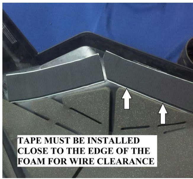
14. Using the picture as a guide, cut the hook and loop tape so it will fit as shown.
