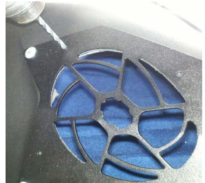
11. Using a 1/8" or #30 drill bit, drill through the side panel using the remaining 4 small holes as a guide.
