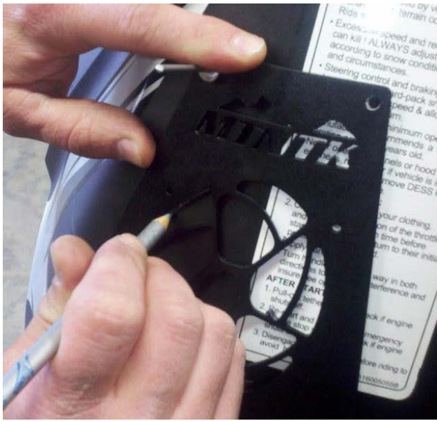
6. Using a silver pencil, scratch awl, or marker, mark the location of the center hole.
