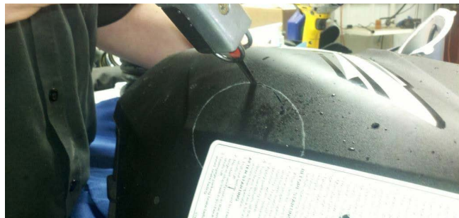
9. Drill a start hole and cut out the marked hole.
