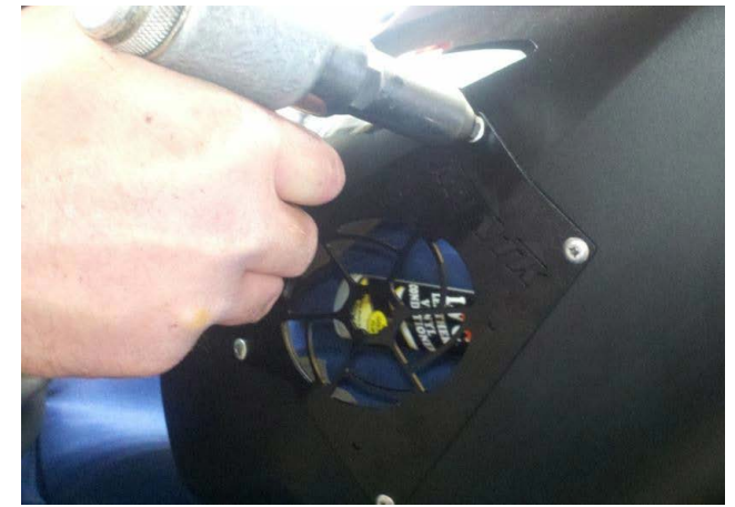
10. Clean up the hole using a rotary tool and or a de-burring tool. Read your warning sticker completely and commit to memory. Remove warning stickers and clean panel of glue residue. If you can not remember what the warning sticker said then be responsible and order new warning decal to install on your sled because it will remind you to not be stupid. Rivet face plate onto side panel using the 3/16" expanding rivets.
