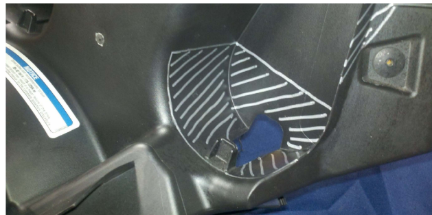
16. Remove spare belt from clutch cover and mark as shown. Take care to reference from the picture to ensure you know what to cut. Lined area is to be removed.
