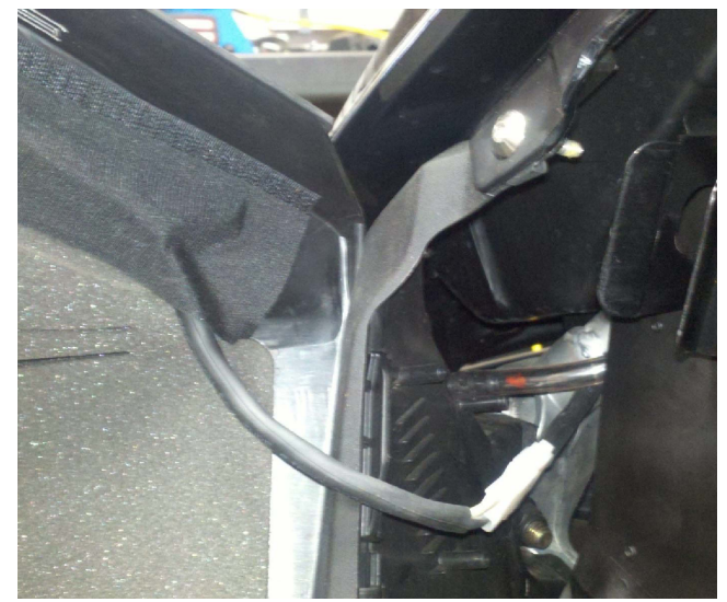
19. Reinstall the clutch cover. Ensure the wires are placed as shown connected and the side panel is installed properly. Check the fit of the panel when closed. It should require a small amount of pressure to snap the cover over the upper side panel hook.
