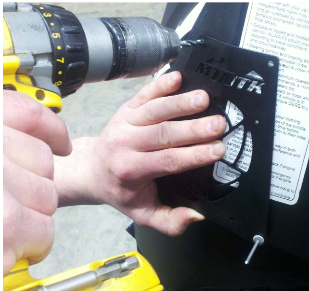
5. Drill (4) 3/6" holes in the outer (4) holes of the face plate through the panel. Start with one hole and place a rivet in the hole temporarily to hold it while moving to the next hole.
