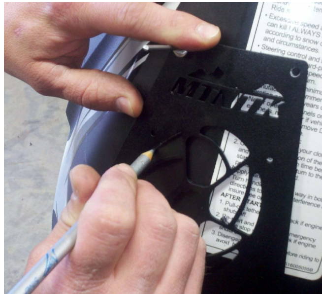
6. Using a silver pencil, scratch awl, or marker, mark the location of the center hole.
