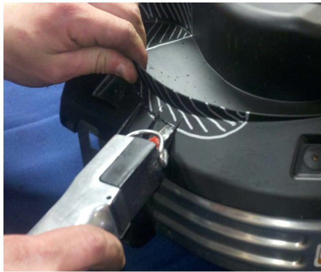
17. Using the saw remove the pieces carefully and deliberately. The plastic has a gummy consistency when cut and using a small amount of an aerosol lubricant will help. Hold the saw horizontal and cut through both faces of the cover at the same time. Remember you can always cut more off if it doesn't fit right!
