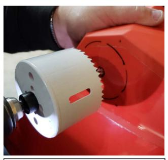
4. Using a silver marker or pen, Mark the center of the fan openings. Remove face plate and rivets. Using a 3" hole saw, cut out the fan opening using the traced out lines as a guide. De-bur the holes you have drilled.
