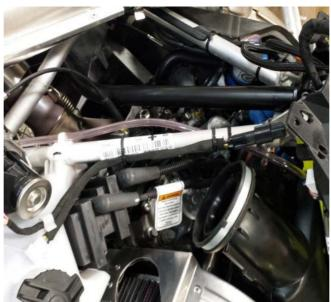
2. Route extension harness down and over the structure tube and onto the top of the oil tank. Replace the hood and gauge console. Reconnect the headlights and gauge console connectors back together.
