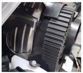
8. Trim the spare belt plastic cover on the clutch cover as shown. Start by cutting the top part off in line with the bracket previously installed. Then carefully grind down the lower part of the plastic cover so the Blow Hole will clear the plastic cover. De-burr all sharp edges.
