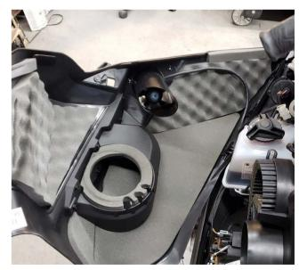
5. Remove foam from inside of your panel. Rivet Blow Hole in place with 3/16" expanding rivets.
