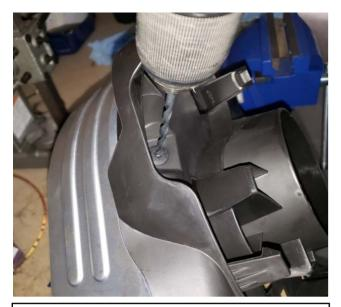
6. Remove clutch cover from machine. Drill out the large head rivet on plastic shroud as shown.
