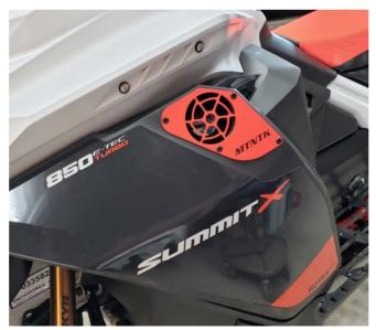
3. Hold face plate up to PTO side panel. Align top and back corner edges as shown. Using a silver marker or pen, mark holes to be drilled. Drill out the marked 3/16" holes. Insert rivets one at a time to hold the face plate in place.
