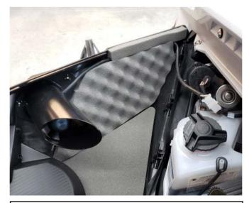
9. Route Blow Hole wire away from clutches and plug into white accessory harness connector.
