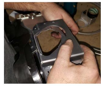
7. Slip the bracket in between the aluminum clutch cover and the black shroud. Align bracket with hole of large head rivet previously drilled. Mark holes to be drilled out. Using bracket as a guide, cut aluminum clutch cover as shown. Install remaining 6 rivets with 2 being installed from the inside-out as shown.
