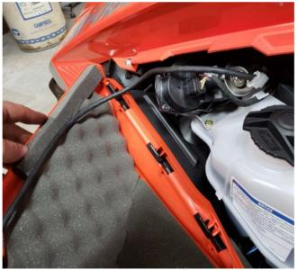
9. Route Blow Hole wire away from clutches and plug into white harness connector.
