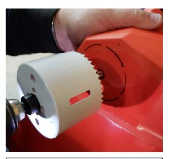
4. Using a silver marker or pen, mark the center of the fan opening. Remove face plate and rivets. Using a 3" hole saw, cut out the fa opening using the traced out lines as a guide. De-bur the holes you have drilled.
