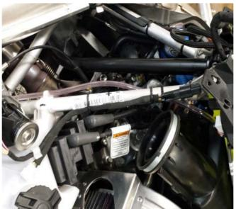
2. Route extension harness down and over the structure tube and onto the top of oil tank. Replace the hood and gauge console. Reconnect the headlights, gauge console, and air temp connectors back together.
