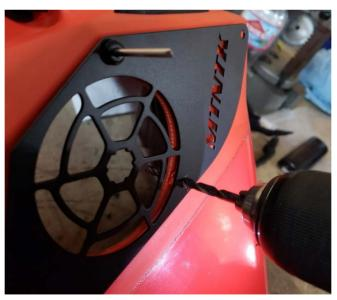
3. Hold face plate up to PTO side panel. Align top and back corner edges as shown. Using a silver marker or pen, mark holes to be drilled. Drill out the marked 3/16" holes. Insert rivets one at a time to hold the face plate in place.
