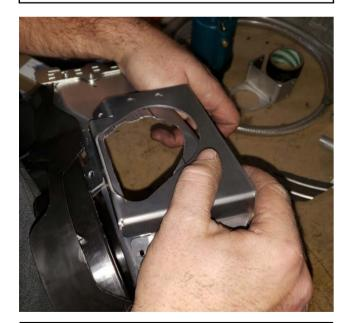
7. Slip the bracket in between the aluminum clutch cover and the black shroud. Align bracket with hole of large head rivet previously drilled. Mark holes to be drilled out.
