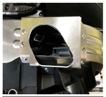
8. Using bracket as a guide, cut aluminum clutch cover as shown, Install remaining 6 rivets with 2 being installed from the inside – out a shown.
