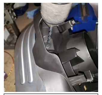
6. Remove clutch cover from machine. Drill out the large head rivet on plastic shrouds as shown.
