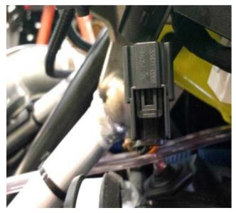
1. Remove side panels, gauge console, hood, and the glove compartment. Find the accessory plug connection site on the PTO side and route the Blow Hole extension harness to the Factory Accessory plug.
