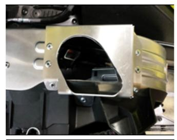
9. Using bracket as a guide, only cut aluminum clutch cover as shown. De-bur everything when finished cutting. Plug the Blow Hole into the extension harness when reinstalling the clutch cover. Clean the clutch compartment of any debris. This is also a good time to verify clutch components have not been damaged...
