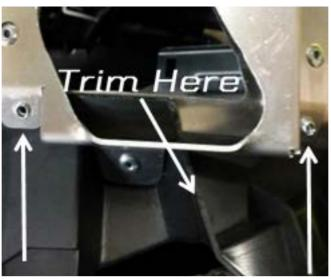
8. You will have to trim the plastic cover as shown. Install remaining 6 rivets with 2 being installed from the inside – out as shown.
