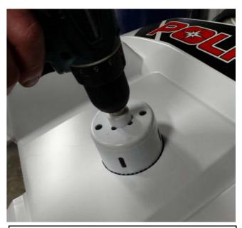
4. Using a silver marker or pen, mark the center of the fan opening. Remove face plate and rivets. Using a 3" holes aw, cut out the fan opening using the center lines as a guide. Debur the holes you have drilled.
