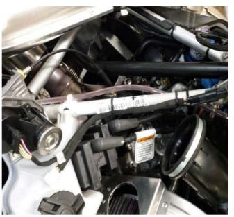
2. Route extension harness down and over the structure tube and onto the top of the oil tank. Replace the hood and gauge console. Reconnect the headlights, gauge console and air temp connectors back together.
