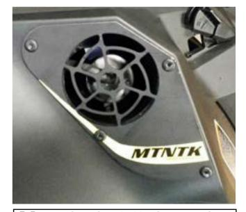
5. Remove foam from inside of your panel. Rivet Blow Hole in place with 3/16" expanding rivets.
