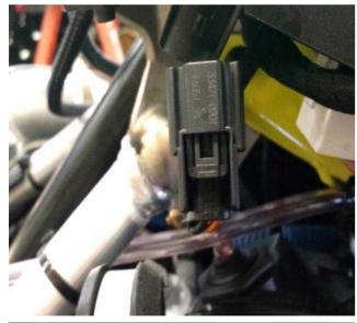
1. Remove side panels, gauge console, hood, and glove compartment cover. Find connection site on the left -hand side near the hand warmer switch under the console. Route Blow Hole extension harness to the connection port.
