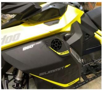
3. Hold face plate up to PTO side panel. Align top and back corner edges as shown. Using a sliver marker or pen, mark holes to be drilled. Drill out the marked 3/16" holes and insert rivets one at a time to hold face plate in place.
