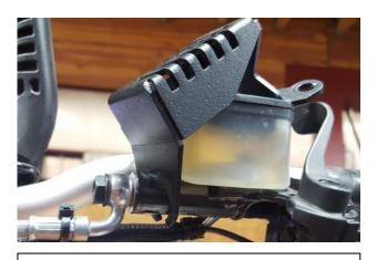
3. Slip reservoir cover over brake line and on top of brake reservoir as shown.
