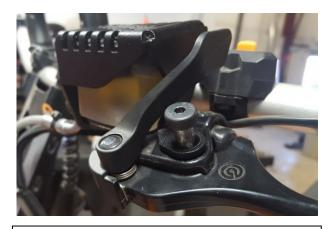
4. Install included brake lever bolt. Tighten remaining mounting bolt. This may fit tight.
