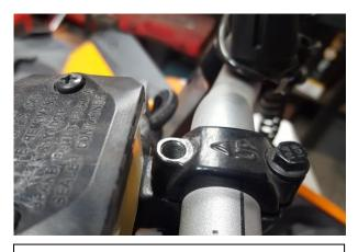
2. Remove the brake reservoir clamp bolt.
