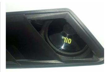
15. Cut the left hand panel upper vent as shown in picture to allow clearance for the oil tank cap. There is a natural line that can
