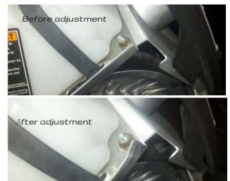
14. The oil tank mount plate/clutch shroud requires a slight adjustment. Bend it over as shown in the photo. A hammer sounds a little severe but it just requires a slight adjustment to make everything fit properly.
