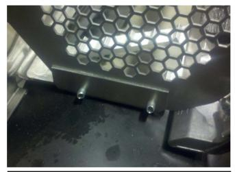
2.2. B. Cut the bottom 1" off of the original kick plate that was removed in step 2. See photo. C. Loosely install new kick plate and the 1" piece you cut off into position. Holding the 1" piece up against the running board, use a sharpie marker or equivalent to mark the position of the 2 rivet holes through new kick plate to the 1" piece. Remove and drill marked holes. Rivet onto the end of the new kick plate. See photo.
