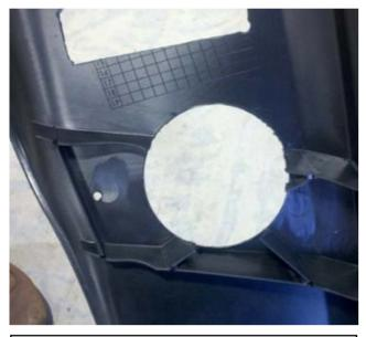
5. Drill hole with 3" hole saw or equivalent. It will go through the ribs on the back side of panel. Also cut out the upper vent as previously marked.
