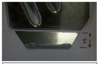
2.1. Remove left hand kick plate by grinding, drilling or shearing off stock rivets. Try not to damage the holes by elongating them during the removal process. Using a pin punch to push the mandrel out of the center of the rivet greatly helps in the drilling process as the mandrel is harder than the rivet.
