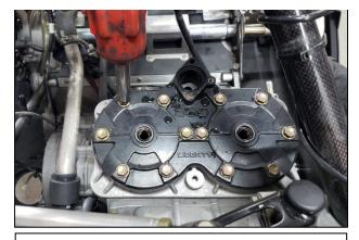
2. Remove spark plugs, head bolts and thermostat housing. Remove head shell from cylinder head. Remove thermostat bleed screw from the top of the thermostat housing.
