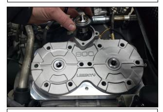
9. Place updated thermostat into head shell as shown. Install thermostat housing onto cylinder head shell. Install Engine Coolant Hose.
