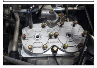
8. Install new head shell. Bolt cylinder head down to cylinder. Torque bolts to 25 ft/lbs. Install DET Sensor and torque to 10 ft/lbs.
