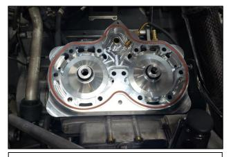
6. Install cylinder head onto cylinder. Be sure gaskets do not move out of place.
