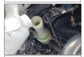
11. Fill coolant bottle. Open bleed screw & bleed coolant system. Start Machine and check for leaks. Continue filling until air bubbles are gone.
