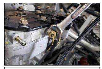
1. Remove hood, side panels, consoles, and drain all the coolant from inside the motor. Remove DET Sensor, Coolant Temp Sensor & all attached coolant lines from the cylinder head.
