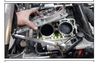
3. Remove cylinder head. It is recommended, but not required, to replace all O-Rings.
