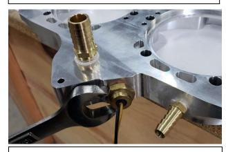
4. Using thread sealant, install included coolant fittings & Thermostat Sensor into MTNTK head.
