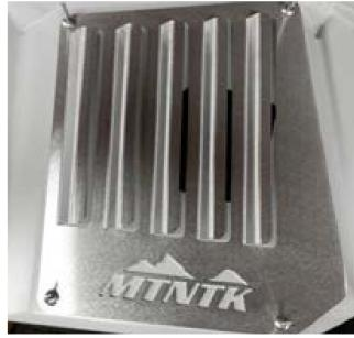
11. Install the vent plate to match body lines of the panel. Mark first, then drill and install the four aluminum expanding rivets as shown.
