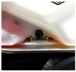
1. Start by removing the left hand side panel. Remove the oil tank retaining bolt. Save the flat washer and discard the bolt.
