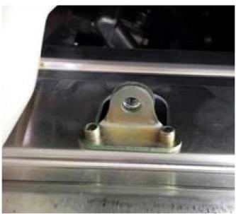
2. Using a 3/16" drill bit, carefully remove the rivets and bracket and discard both.
