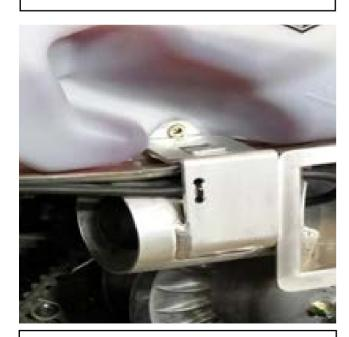
7. Mount the Blow Hole and route the wires as shown so there is no slack above the primary clutch. Plug into the factory DC power port.
