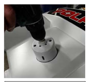
10. Drill a pilot hole in the center of the X, then using a  $\mathbf{3}$ " hole saw, drill a hole.
