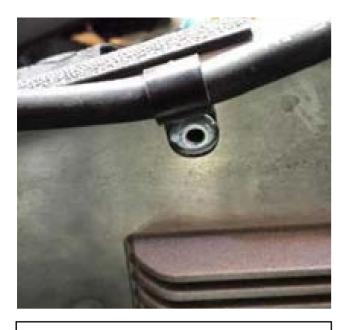
6. Place the wire holder onto the Blow Hole wire then rivet into place as shown.
