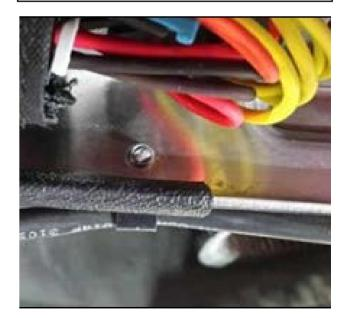
5. Drill a 3/16" hole in the aluminum shelf measuring 3" back from the front of the shelf.
