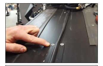
4. Use the taillight wire guide to mark new locations for the rivets down the center. This will ensures correct location. Make sure the front is centered in the tunnel before marking. Insert Tunnel Cooler through the drilled holes.
