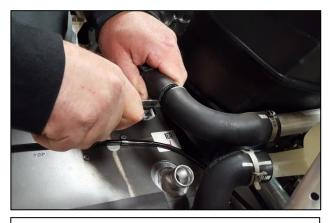
6. Use the Hose Cut Guide to cut the hose which comes off the cylinder head thermostat. Install and secure with hose clamps. ('11-'15 SEE STEP 7)
