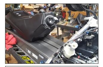
1. Remove rear suspension, track, seat, and fuel tank. Driveshaft & track removal not required but recommended. Remove left hand cooler hose and drain the cooling system. A clean shop vacuum set up for liquid works best.
