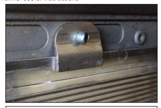
5. Secure the cooler with one rivet in the front and back. Align remaining rivets and secure. Rivet clamp plates under the tunnel as shown.
