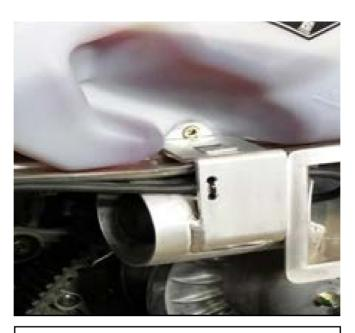
8. Mount Blow Hole as shown. Install side panel and remove outer graphic from panel. Wait for imprint to appear in panel foam. This will be a guide to drill out the outlet for the Blow Hole.
