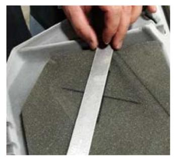
9. Using a straight edge, draw a line from corner to corner within the imprint shown.
