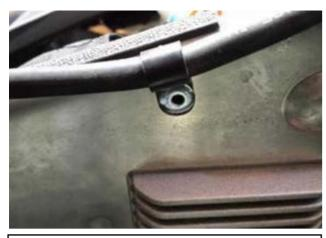
6. Place wire holder onto the Blow Hole wire then rivet into place as shown.
