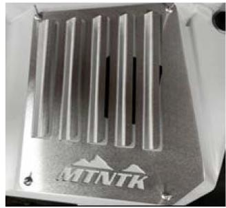
11. Install the vent plate to match body lines of the panel. Mark first, then drill and install the four aluminum expanding rivets as shown.
