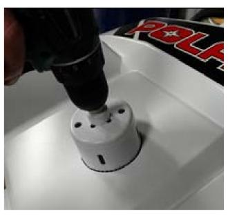
10. Drill a pilot hole in the center of the X, then using a 3" hole saw, drill a hole.
