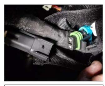
7. Route harness up the frame to harness bag under the center console. Locate plug cap labeled **RCA ACCY POWER.** Remove cap and plug Blow Hole into Accy Plug as shown.
