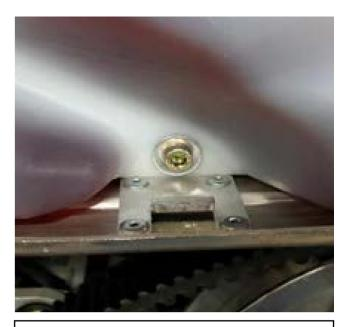
4. Install the previously removed flat washer onto the new bolt and install into the new bracket, holding the oil tank in place.
