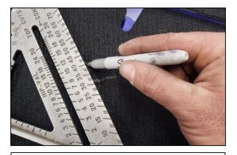
4. Remove the side panel. Your Blow Hole should have left an imprint in the side panel foam. Using a straight edge, quickly mark the center of your Blow Hole imprint onto the foam. This mark is to be used as a reference only!
