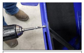
1. Remove the side panel from the clutch side of the snowmobile. Remove the front Torx Screw from the side panel support then Using a ¼" Drill Bit, drill out the side panel support as shown.
