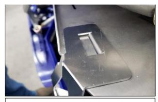
2. Slide the top end of the Blow Hole assembly into the top slot of the clutch cover as shown.
