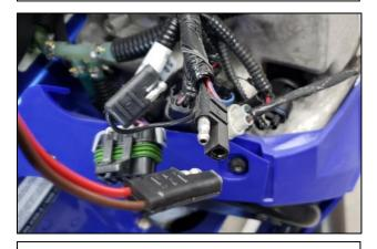
10. Route the Blow Hole wiring harness up towards the steering post, down the side of the gas tank towards the oil bottle. Remove the stock accessory plug cap and plug it into the stock accessory plug.
