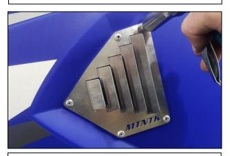
9. Using a 3/16" Drill Bit, drill out these previously marked holes. Using a rivet gun, rivet the Blow Hole Plate to the outside of the side panel as shown.
