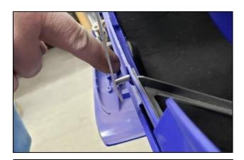
3. Slide the bottom locating pin of the Blow Hole assembly into the previously drilled ¼" hole located at the side panel plastic support bracket. With the Blow Hole Assembly installed, install the side panel back onto the Clutch Side of your snowmobile. Let your sled sit for at least 30 min.
