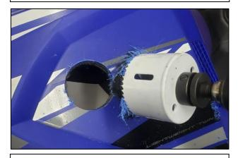
7. Using a 3" Hole Saw, drill out the location of your new pilot hole. Deburr and clean all the shavings from around the hole.
