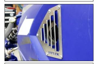
8. Align the Blow Hole Plate so the 3" hole is centered inside the plate's louvers. Once aligned, mark the 3/16" Holes surrounding the Plate.
