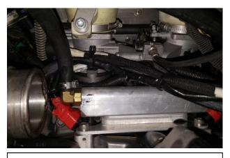
4. Remove Brass 90° Barb fittings w/O-Rings from stock fuel rail and install on updated fuel rail. Do not tighten. Install injectors w/O-Rings into cylinder. PTO wire is longer than MAG. Install Updated Fuel Rail onto injectors using supplied 6MMx1.0x16mm Bolts
