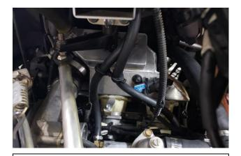
5. Install Fuel lines onto Updated Fuel Rail. PTO side is White, MAG side is Black. Crimp Oetiker Clamps onto the 90° Brass fittings, away from Silicone Turbo Intake Hose. Route fuel lines up to gas tank. Tighten the Brass 90° Barb fittings onto fuel rail. \*Routing of these fuel lines is crucial. Improper routing could result in fire\*
