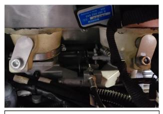
3. Using the supplied 6MMx1.0x20mm Bolts, move the aluminum injector plugs from the cylinder into the white charge box adapters. Don't forget to install the Injector O-Rings onto the aluminum injector plugs and install the Green O-Rings into the Charge Box Adapters and Cylinder Injector Holes
