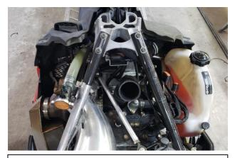
1. Remove side panels, hood, center console, intake console, and the silicone turbo intake hose. Removal of TurboCharger is not required.
