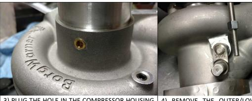
3) PLUG THE HOLE IN THE COMPRESSOR HOUSING WITH THE 1/8" BRASS PIPE PLUG. USE THREAD SEALANT AND TIGHTEN.
