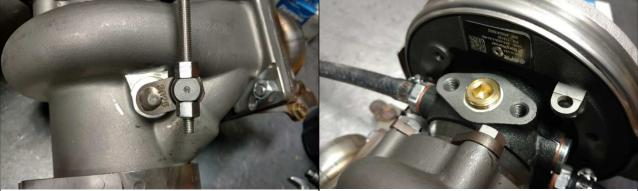
9) REINSTALL THE WASTEGATE ROD AND TAKE CARE NOT TO MOVE THE INNER/UPPER NUT SO YOUR BOOST LEVEL WILL REMAIN THE SAME. 10) TURN THE TURBOCHARGER OVER AND FILL THE CENTER SECTION FROM THE BOTTOM DRAIN HOLE WITH CLEAN TWO STROKE OIL LEAVING A 1/2" AIR SPACE FROM THE TOP. APPLY THREAD SEALANT AND INSTALL THE 3/8" BRASS PLUG.
