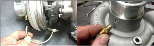
1) REMOVE MUFFLER AND TURBOCHARGER FROM2) REMOVE THSLED. REMOVE THE OIL LINE LOOP TUBE FROMFROM THE ITHE TURBO CENTER SECTION/COMPRESSORHOUSING.HOUSING.HOUSING.
