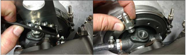
5) USING A 4MM ALLEN L-WRENCH REMOVE THE 3 SCREWS HOLDING THE WASTEGATE BRACKET AND REMOVE IT.
