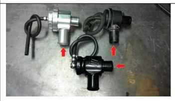
8) INSTALL BLOW OFF VALVE WITH THE ARROW FITTING TO THE CHARGE TUBE. DEPENDING ON WHICH VALVE YOU HAVE WILL DETERMINE THE PROPER HOSE ROUTING. USE PICTURE ABOVE. TIGHTEN ALL CONNECTIONS
