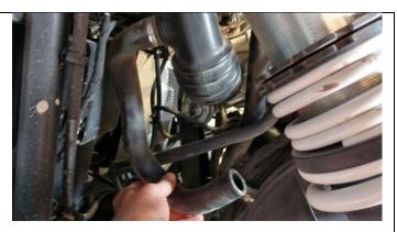
2) CUT OFF AND REMOVE THE CLAMP SECURING THE RECIRCULATION HOSE TO THE BOTTOM OF THE BLOW OFF VALVE AS SHOWN.
