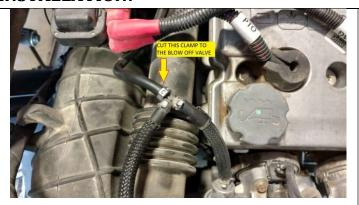
1) LOOSEN AND REMOVE THE CLAMP SECURING THE CHARGE TUBE TO THE TURBOCHARGER AND THE CLAMP AT THE REAR ON THE THROTTLE BODY. IT IS NOT REQUIRED, BUT REMOVAL OF THE MUFFLER AND REAR SHIELD PANEL IS HELPFUL IN GETTING TO THE CLAMP. 7/16" DEEP SOCKET REQUIRED.
