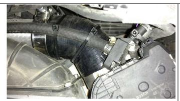
11) SECURE THE BOOST SENSOR AND HOSE WITH PROVIDED NYLON CABLE TIES.
