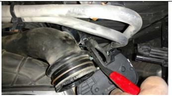
4) PULL OUT THE CHARGE TUBE JUST FAR ENOUGH TO CUT OFF THE NYLON TIES SECURING THE WIRE TO THE SENSOR. ENSURE YOU ARE NOT PULLING ON THE WIRES TO THE BOOST SENSOR. DO NOT REMOVE THE SENSOR PLUG! IT IS A DOUBLE LOCK DESIGN AND IS VERY DIFFICULT TO REMOVE WITHOUT BREAKING IT!
