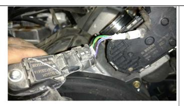
5) USING A #25 TORX REMOVE THE SCREW SECURING THE BOOST SENSOR AND REMOVE IT FROM THE CHARGE TUBE. JUST LET IT HANG OUT FOR A MINUTE. INSERT THE CHARGE TUBE AND SECURE IN PLACE STARTING WITH THE CONNECTION ON THE TURBO. WORK YOUR WAY BACK TIGHTENING THE CLAMPS AND ADJUSTING THE SILICONE TO FIT.
