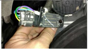
10) PLACE A NYLON TIE ON THE WIRE AND SECURE AS SHOWN. THIS WILL PREVENT WIRE BREAKAGE.
