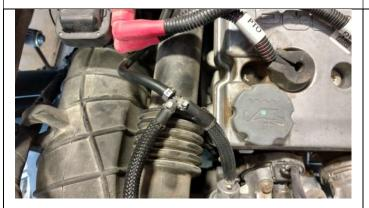
9) CONNECT THE HOSE FOR THE BLOW OFF VALVE AND SECURE WITH OETIKER CLAMP.
