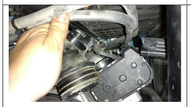
3) WITH CONSIDERABLE EFFORT PULL THE CHARGE TUBE OFF OF THE THROTTLE BODY. ENSURE YOU ARE NOT PULLING ON THE WIRES TO THE BOOST SENSOR. DO NOT REMOVE THE SENSOR PLUG! IT IS A DOUBLE LOCK DESIGN AND IS VERY DIFFICULT TO REMOVE WITHOUT BREAKING IT!
