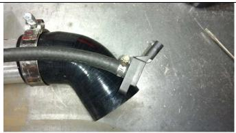
6) INSERT THE BOOST SENSOR INTO THE 3/8" HOSE AND SECURE WITH THE PROVIDED HOSE CLAMP. DON'T OVER TIGHTEN THE CLAMP AND DAMAGE THE SENSOR. (CHARGE TUBE REMOVED FOR CLARITY YOURS IS ON THE VEHICLE)
