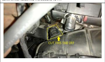
7) TRIM THE SMALL RUBBER TAB ON THE CLUTCH OUTLET DUCT FOR CLEARANCE. INSTALL THE 90 DEGREE RUBBER HOSE WITH THE HOSE POINTING TO THE FRONT OF THE RZR. WAIT TO TIGHTEN THE CLAMP UNTIL THE BLOW OFF VALVE IS INSTALLED AND FIT IS DETERMINIED.
