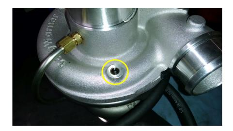
• ROUTE THE SUPPLIED HOSE MAKING SURE THERE ARE NO KINKS, AND THAT IT DOES NOT INTERFERE WITH ANY STEERING OR OTHER LINKAGES.
