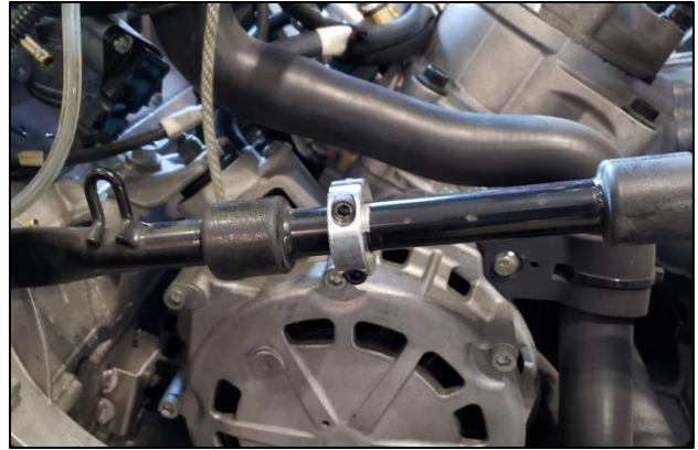
18. Install the included Split Collar up to your mark as shown. This will locate the Turbo brace.
