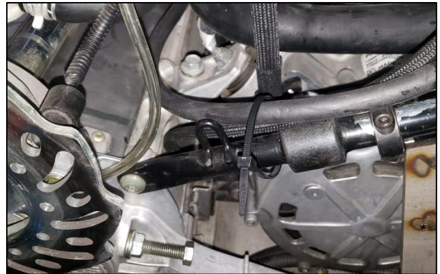
22. Route the MAG coolant line and Turbo Oil Feed Line up to the stock frame brace. Secure with a Zip tie.
