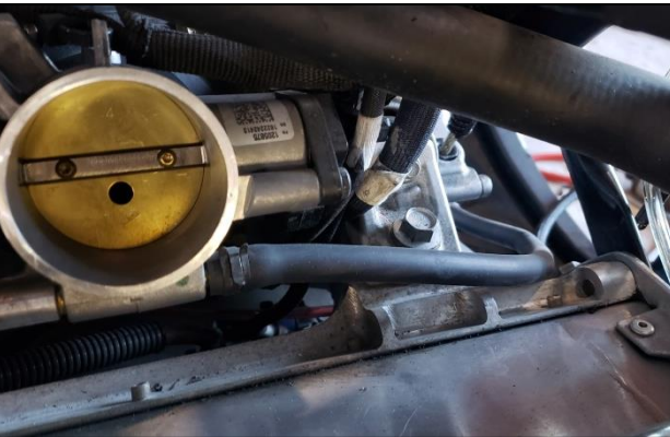
21. Install the included 14" Coolant line onto the MAG Throttle Body coolant fitting.
