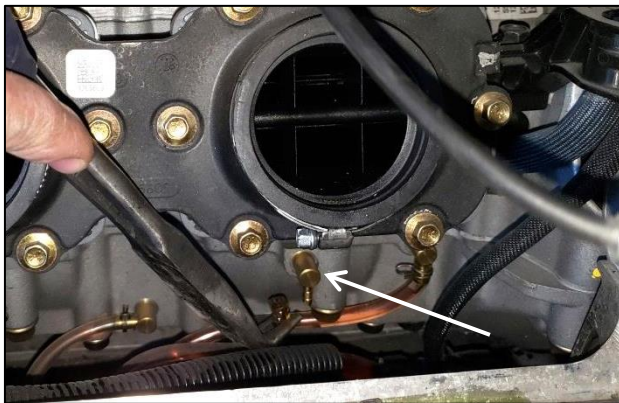
9. Remove the stock MAG Rod Oil line from the MAG Rod Oil Fitting located under the MAG Reed.
