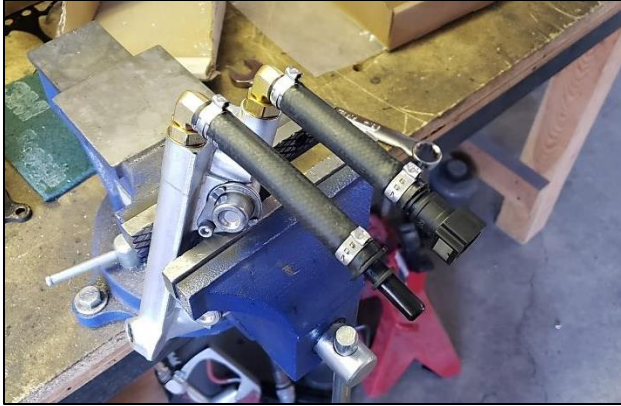
6. Re-connect the turbo fuel line assembly. Do not tighten fittings until fuel rail is installed.
