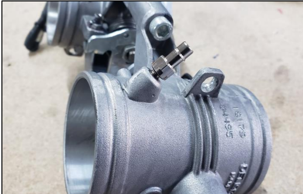
8. Using Red Loctite, install the included boost reference fitting into the PTO throttle body.
