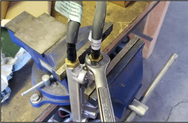
5. Remove stock fuel lines from the stock fuel rail assembly as shown.
