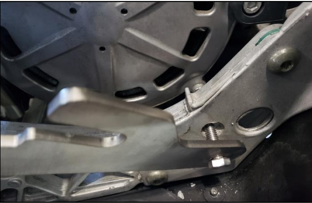
19. Install the Turbo Brace as shown through the frame opening using the included 25mm bolt and placing the 5/16" flat washer on the inside of the frame opening.
