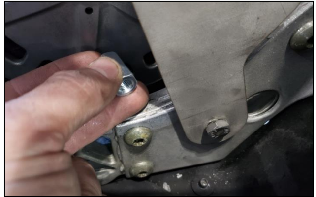
20. Install the included coupler nut and 5/16" washer on the backside of the frame opening to secure the Turbo Brace. Slide brace tightly up against the installed Split Collar. Tighten Bolt.
