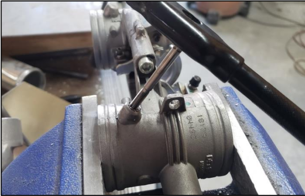
7. Using a 10-32 Tap and #21 Drill bit, carefully drill and tap the PTO Throttle body as shown. Deburr hole and remove all metal shavings from throttle body. Clean throttle body thoroughly.
