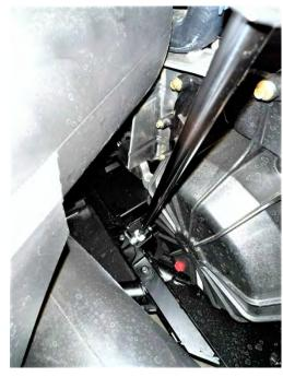
NEXT YOU WILL INSTALL THE BLOWHOLE ASSEMBLY ONTO YOUR MACHINE AS SHOWN IN THE PICTURE BELOW. IT IS EASIEST TO INSTALL THE RUBBER HOSE ONTO THE CLUTCH BOX COVER FIRST AND THEN THE OTHER END OF THE BLOWHOLE ASSEMBLY ONTO THE PLASTIC INTAKE PIPE ON THE MACHINE. BE SURE TO TIGHTEN ALL 3 HOSE CLAMPS.
