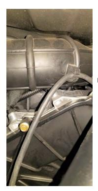
ROUTE THE BLOWHOLE ELECTRICAL WIRE STRAIGHT UP IN FRONT OF THE CLUTCH BOX COVER TO THE ENGINE AIR INTAKE HOSE. INSTALL WIRE INTO HOLDER THAT IS MOLDED INTO HOSE. ROUTE THE WIRE TOWARDS
