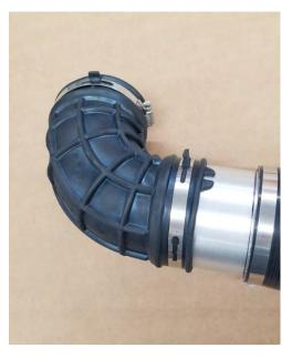
INSTALL PREVIOUSLY REMOVED RUBBER 90 DEGREE HOSE ONTO THE ALUMINUM PIPE ON THE BLOWHOLE ASSEMBLY. LEAVE HOSE CLAMP LOOSE AT THIS TIME TO ALLOW YOU TO ALIGN THE RUBBER BOOT TO THE PROPER POSITION.
