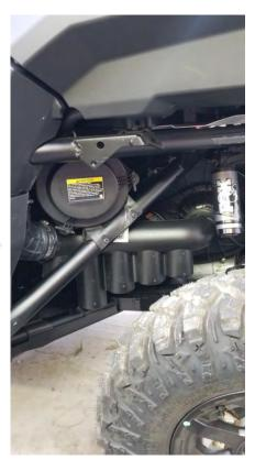
FIRST LOOSEN THE 2 HOSE CLAMPS THAT THE ARROWS ARE POINTING TO IN THE PICTURE TO THE LEFT.
