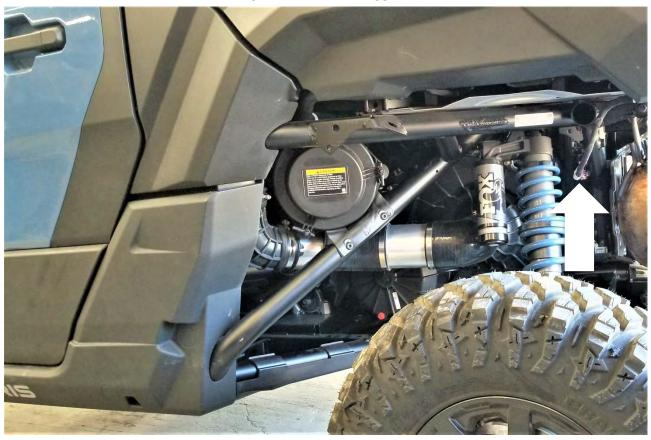
THE ARROW IN THE PICTURE ABOVE IS POINTING TO THE LOCATION OF THE STOCK ELECTRICAL CONNECTOR WHERE THE BLOWHOLE WILL BE PLUGGED INTO.
