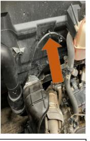
7. After reinstalling the outlet tube, you will use the retaining zip ties included in the kit to retain the power wire and outlet tube as showing in the picture.
