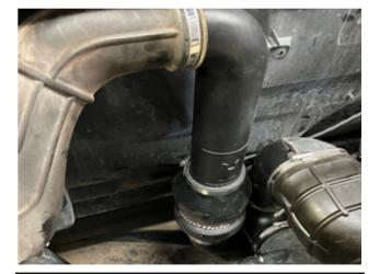
5. Now you will install the Blow Hole into the intake tube. The top half of the tube will flex over out of the way and the Blow Hole can be slid onto the lower half of the tube. Then align the top half of the intake tube and the Blow Hole. Then slide the Blow Hole up onto the top half of the intake tube.
