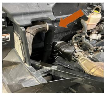
1. The intake and exhaust tubes will be hooked together by a hose clamp. Remove both tubes from the machine assembly.
