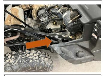
8. You will run the Blow Hole power wire along the cab back wall, behind the coolant overflow reservoir, under the air filter housing to get to the right side of the machine. The power wire will be connected to the taillight harness connector that is located right by the voltage regulator. Unplug the factory taillight connector and plug the Blow Hole connector in line with the factory connector. This will now power the Blow Hole and taillights.
