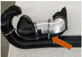
2. Remove the hose clamp holding the tubes together. This hose clamp will not be reused.
