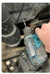
6. You will need to enlarge one hole and drill a new hole that will be 1/4". The picture on the left above shows the hole that needs to be enlarged. This hole will be used to retain the power wire for the Blow Hole.
