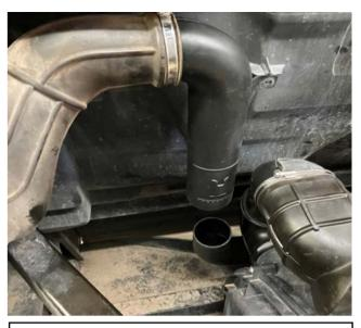
4. Install the bottom half of the intake tube onto the clutch housing first. Next install the exhaust tube onto the clutch housing. Then install the top half of the intake tube into the intake screen boot that is attached to the side of the machine.
