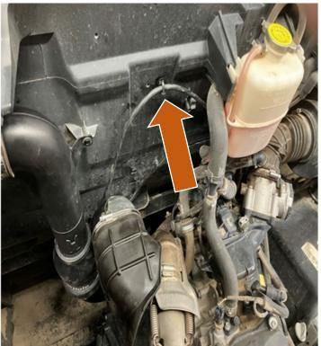
AFTER REINSTALLING THE OUTLET TUBE, YOU WILL USE THE RETAINING ZIP TIES INCLUDED IN THE KIT TO RETAIN THE POWER WIRE AND OUTLET TUBE AS SHOWN IN THE PICTURE.
