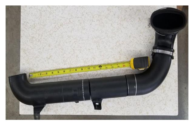
USING THE INTAKE TUBE SHOWN IN THE PICTURE YOU WILL CUT A SECTION OUT OF THE MIDDLE OF THE TUBE. MEASURING FROM THE INSIDE OF THE 90\* BEND, AS SHOWN IN PICTURE, MAKE THE FIRST LINE AT 10" AND A SECOND LINE AT 15.75".
