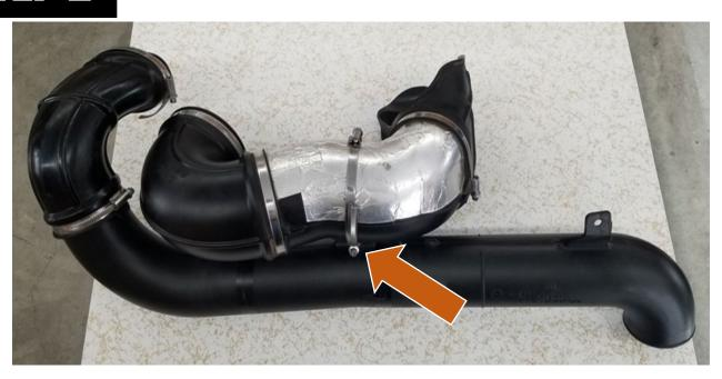
REMOVE THE HOSE CLAMP HOLDING THE TUBES TOGETHER. THIS HOSE CLAMP WILL NOT BE REUSED.
