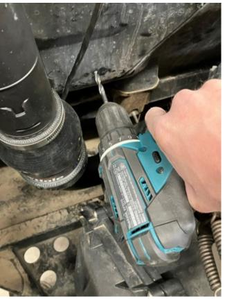
YOU WILL NEED TO ENLARGE ONE HOLE AND DRILL A NEW HOLE THAT WILL BE 1/4". THE PICTURE ON THE LEFT ABOVE SHOWS THE HOLE THAT NEEDS TO BE ENLARGED. THIS HOLE WILL BE USED TO RETAIN THE POWER WIRE FOR THE BLOWHOLE.
