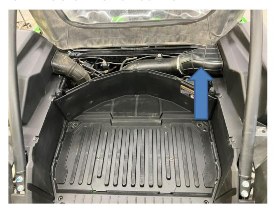
2. REMOVE RUBBER BOOT BETWEEN THE AIR INTAKE HOUSING AND CLUTCH BOX INTAKE TUBE – SEE PICTURE ABOVE – ARROW IS POINTING AT THE RUBBER BOOT
