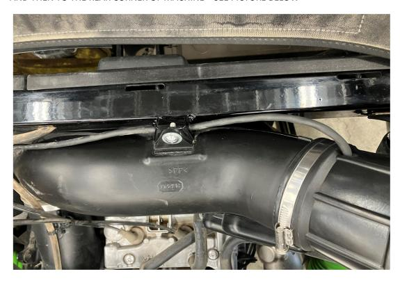
7. THE MACHINE POWER SUPPLY WIRES ARE LOCATED UNDER THE REAR FENDER ON LEFT HAND SIDE — THEY ARE TAPED UP TO THE WIRING HARNESS WITH PLUGS IN THE CONNECTORS
