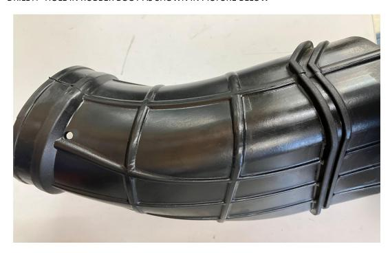
4. INSERT BLOWHOLE WIRE, FROM THE INSIDE OF TUBE, THROUGH THE HOLE THAT YOU JUST DRILLED – INSERT BLOWHOLE ALUMINUM TUBE INTO RUBBER BOOT WITH FAN BLADE INSIDE RUBBER BOOT AS SHOWN BELOW
