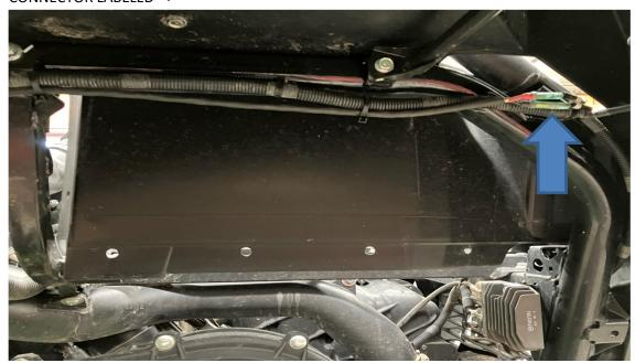
9. TURN THE IGNITION KEY ON, BUT DO NOT START THE ENGINE, AND DOUBLE CHECK THAT THE AIR FROM THE BLOWHOLE IS FLOWING THE CORRECT DIRECTION – THE AIR SHOULD BE BLOWING OUT OF THE OPEN TUBE BY THE EXHAUST – IF IT IS NOT BLOWING OUT THE POWER WIRES ARE CONNECTED WRONG AND NEED TO BE SWITCHED
