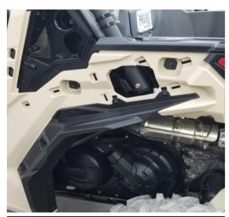
Remove the left rear bed side panel, the clutch intake vent air deflector, and the stock auxiliary air intake tube. The foam on backside of deflector will need to be removed.
