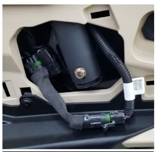
5. Next you run the blowhole wire up to the inside of the left hand rear fender. The connector seen in the picture above is for the left hand tail light. This is where the blowhole will be plugged into. Unplug the tail light and plug the blowhole in line with the tail light.
