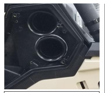
3. Insert the end of the 3"  $90^{\circ}$  silicone hose into the enlarged hole. Fold the silicone in on itself and insert the hose into the hole, then unfold the silicone to fit tight into the hole.
