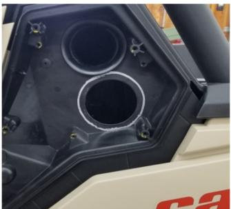
2. Draw a 3.5" circle around the stock intake opening. The silicone hose supplied with the Blow Hole requires the bigger opening to fit properly.
