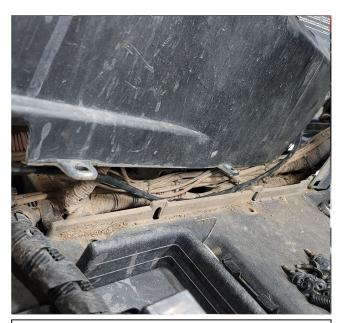
4. Route the Blow Hole wire harness under the center console and up behind the dash. Make sure to route the wire away from the drive system. Secure harness using zip ties.
