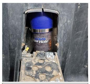
2. Install the Blow Hole into the access panel. Slide the 90° silicone over the upper CVT Intake Duct. (See Step 3 Below)
