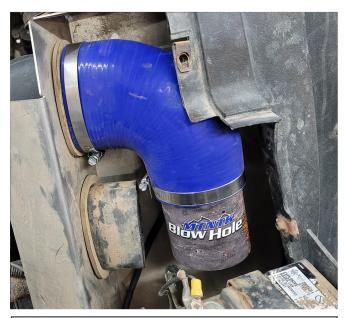
3. Tighten the clamp onto the CVT intake duct.
