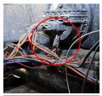
5. Locate the 2-Wire Accessory Plug under the dash. It is located directly behind the speedometer. Plug the Blow Hole Harness into this Accessory Plug.
