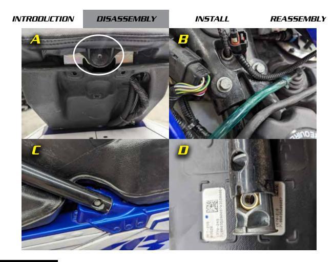
Remove Seat and Rear Spar Tubes
