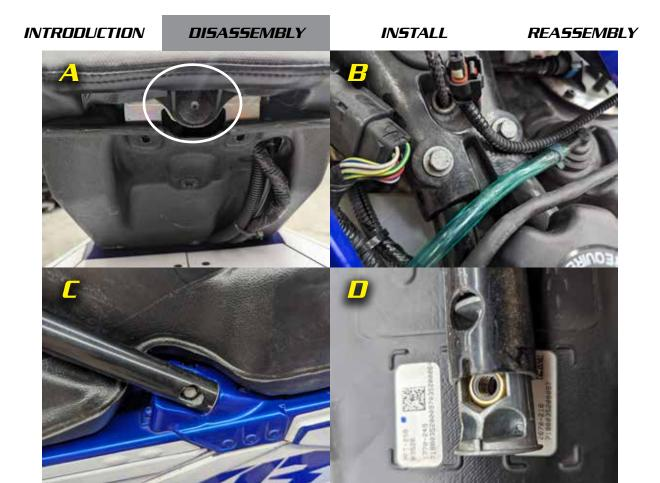
Remove Seat and Rear Spar Tubes
