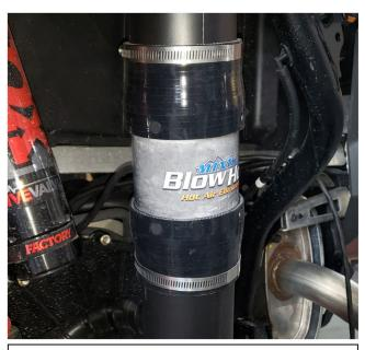
5. Install the Blow Hole in line with the cut intake tube as shown. Keep clamps loose. Install intake tube into stock location on the clutch cover. Once aligned, tighten clamps.
