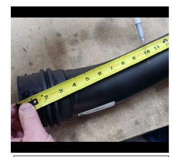
2. Measure 10" from the straight end of the intake tube and mark using a white marker.
