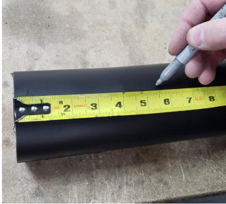
4. Measure 5 1/2" from the cut you just made towards the bottom of the intake tube. Mark using a white marker. Cut completly through the intake tube at this mark.
