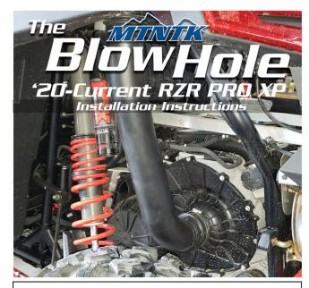
1. Locate the clutch housing intake tube and loosen clamp on clutch cover. Then remove intake tube from both intake and clutch cover.
