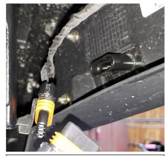
6. Route wiring harness along the bed so it is up and out of the way. Plug directly into the taillight as shown. Be sure the wires will not rub, chafe, or melt. Use zip ties to secure wiring harness.
