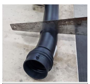
3. Cut completly through the intake tube at the correct mark. Be sure to keep your blade straight so you can achieve a straight cut.
